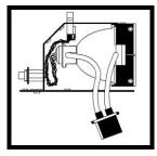
7. Locate the Power connector with two leads and connect it to its mate located on the bottom of the lamp-housing wall.
