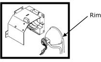
Make sure the middle of the lamp is in position to fit into the spring clamp. Slide the lamp until it snaps into the spring clamp. The leading edge of the reflector should fit snugly into the lamp holder recess.
